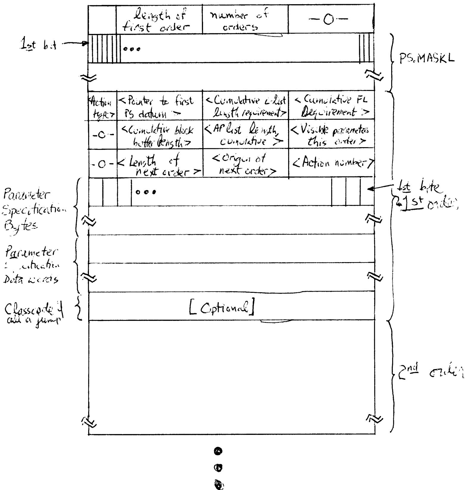
Parameter-type bit mask: 0=datum, 1=capability or block (which also uses two words in the AP list)
