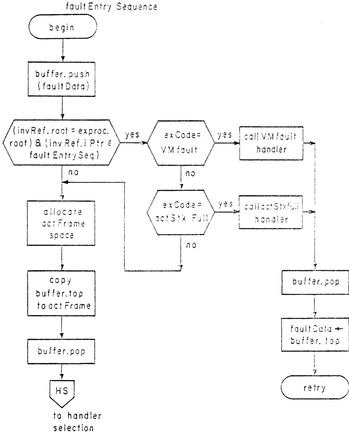
figure 4-4: Fault Entry (modified)
