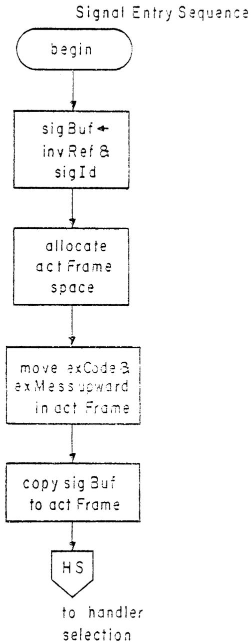
figure 4-6: Signal Entry Sequence
