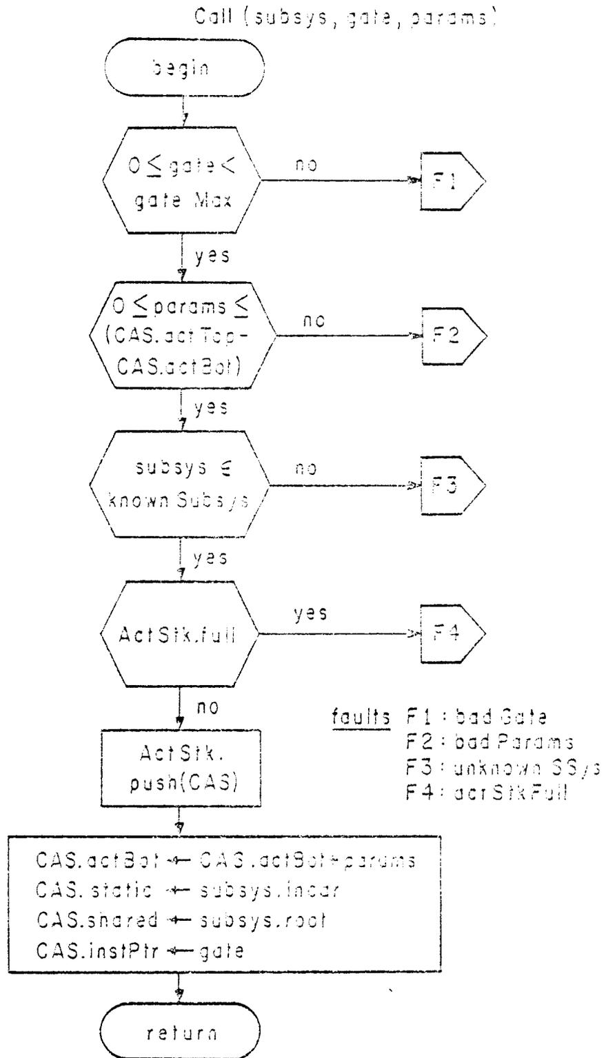
Figure 3-6: Subsystem Call -- Algorithm
