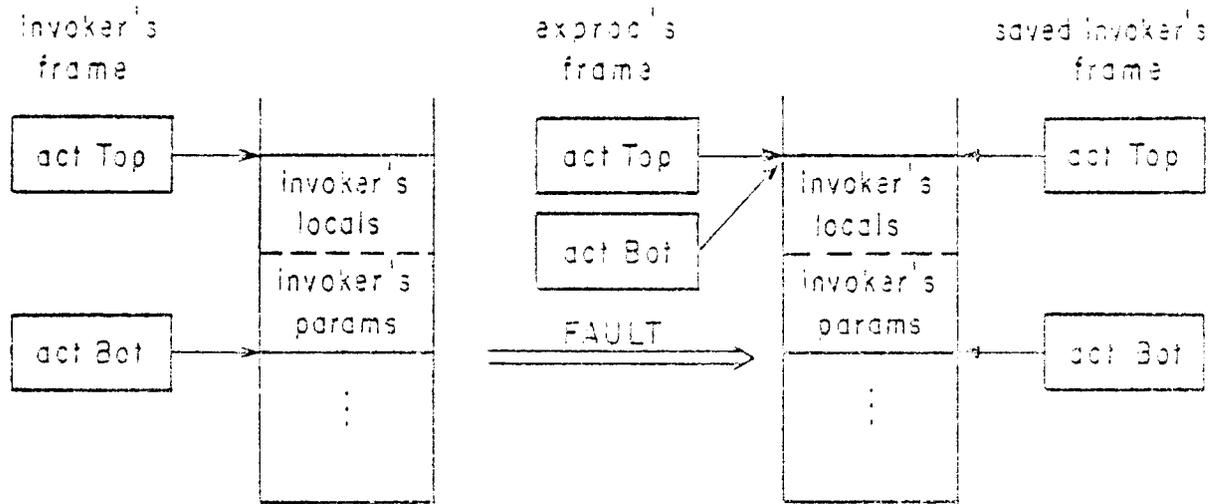
Figure 3-13: Basic Fault -- Activation Frame
