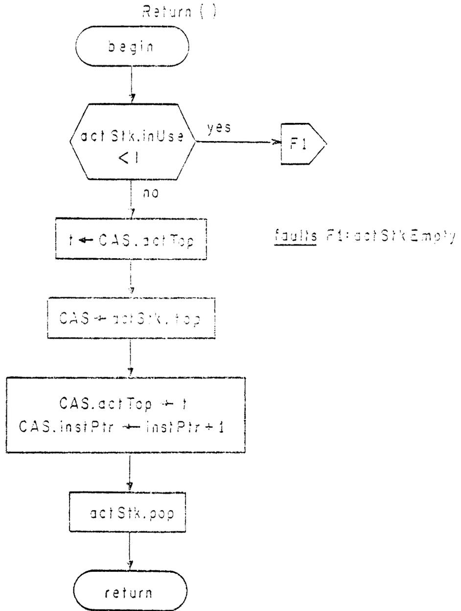
Figure 3-9: Substack Return -- Algorithm
