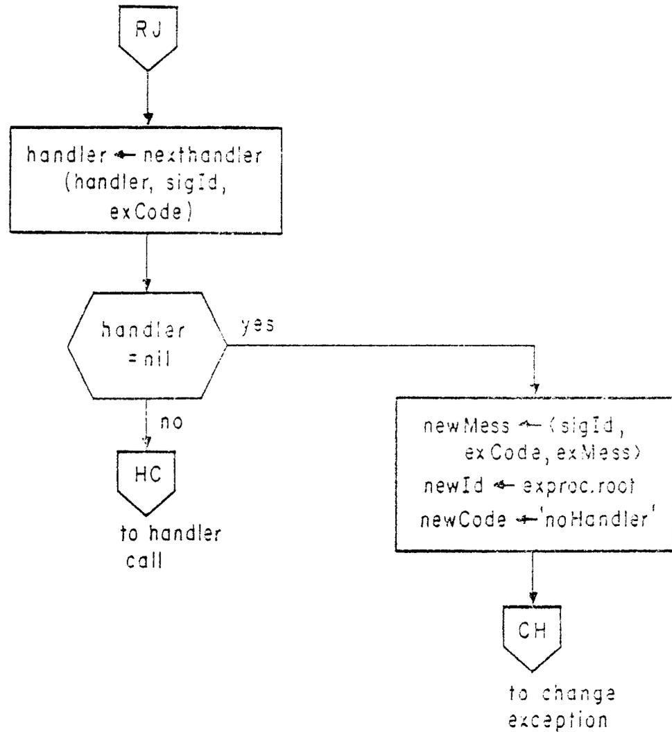
figure 4-23: Reject Termination
