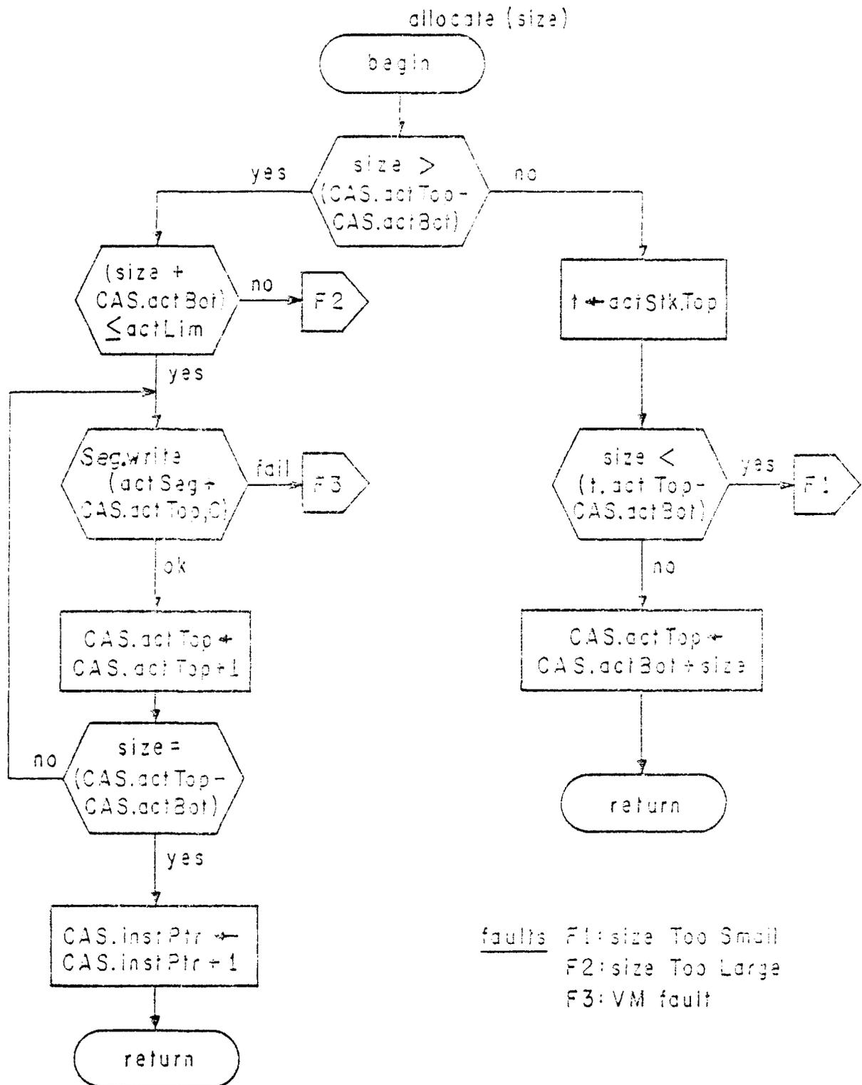
Figure 3-11: Allocate Algorithm
