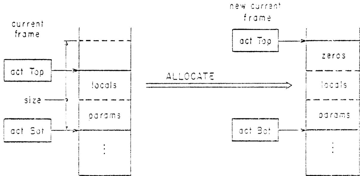
Figure 3-10: Allocate Activation Frame
