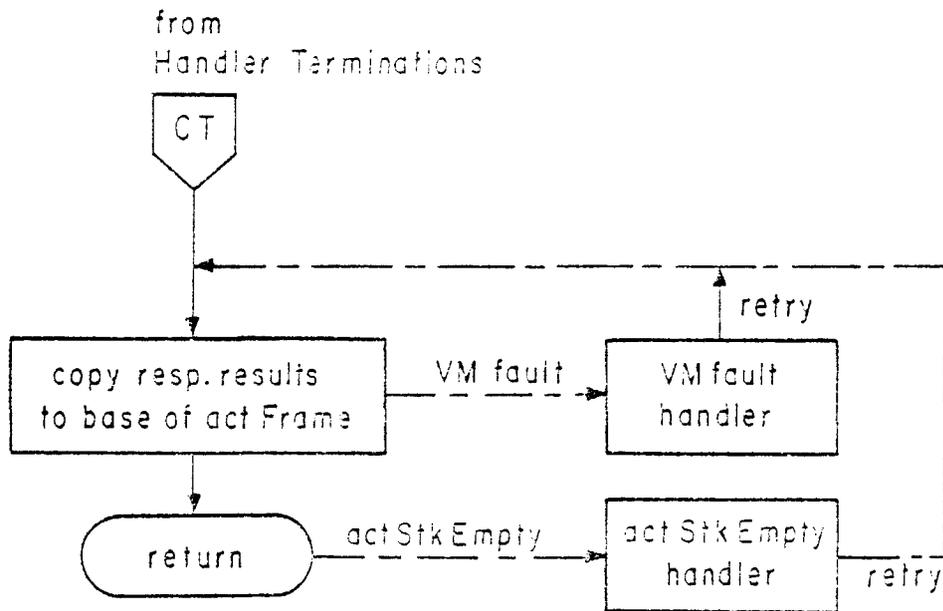
figure 4-15: Continuous Termination
