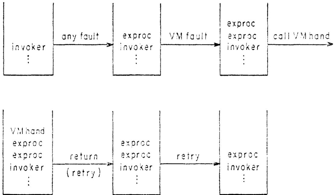
figure 4-3: Fault Entry -- Virtual Memory Fault
