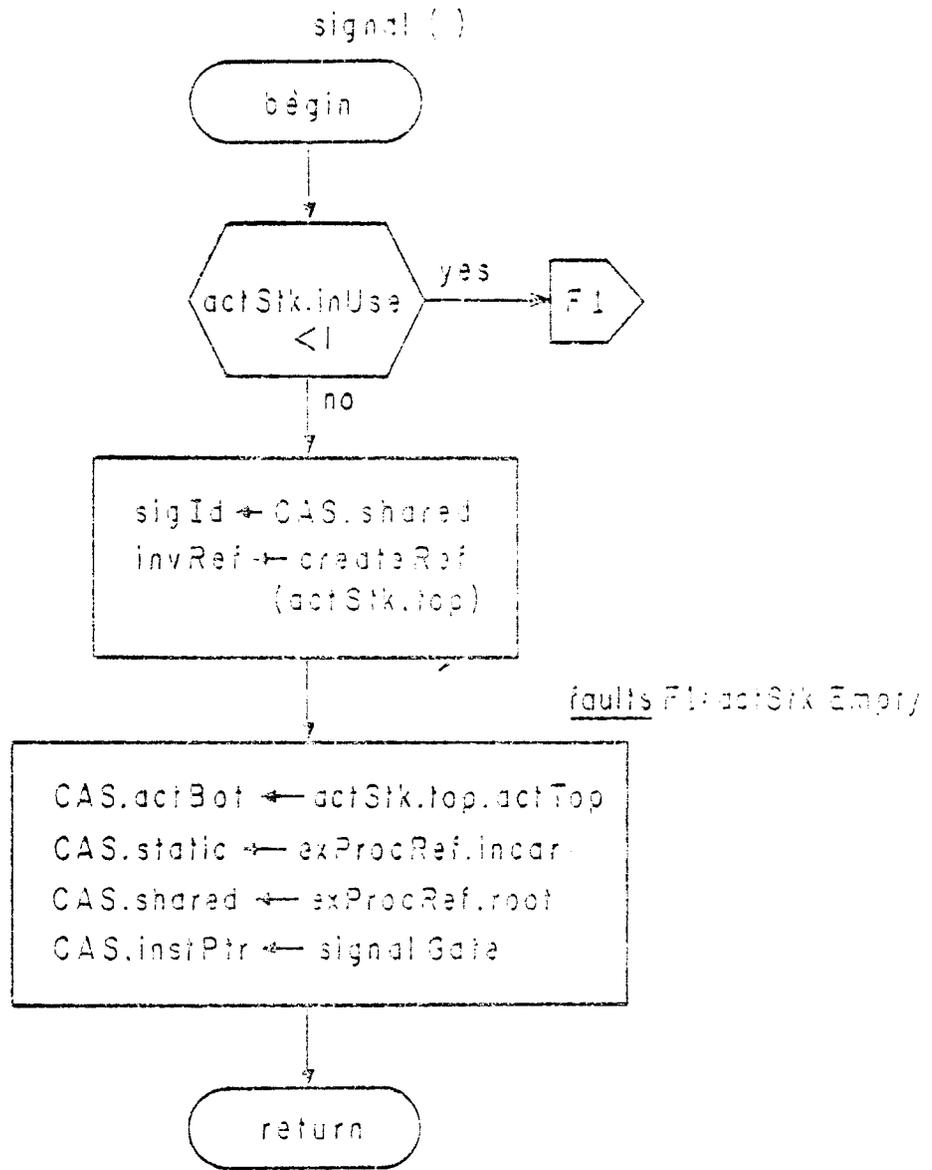
figure 3-13: Signal -- Algorithm
