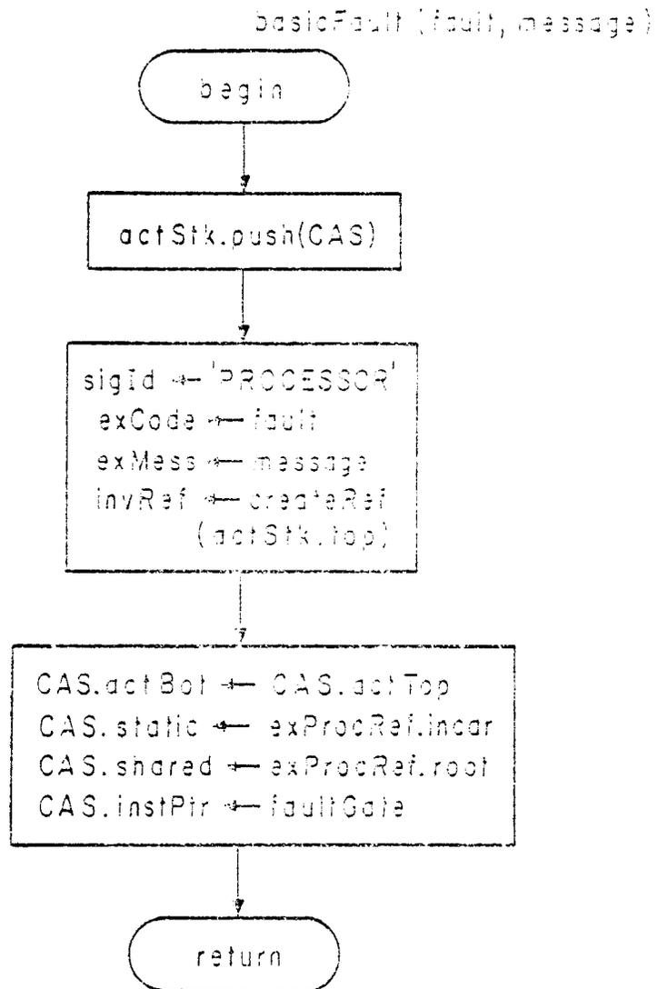
figure 3-15: Basic Fault -- Algorithm
