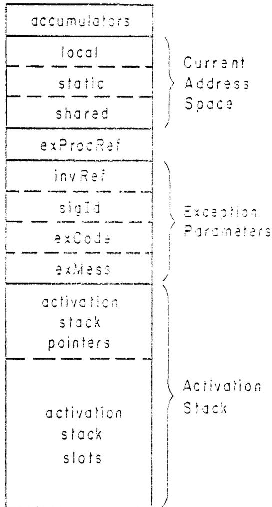
figure 3-12: The Process Base (Augmented)
