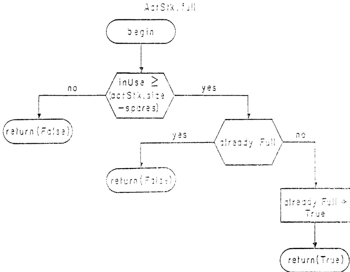
Figure 3-25: Activation Stack Full Test
