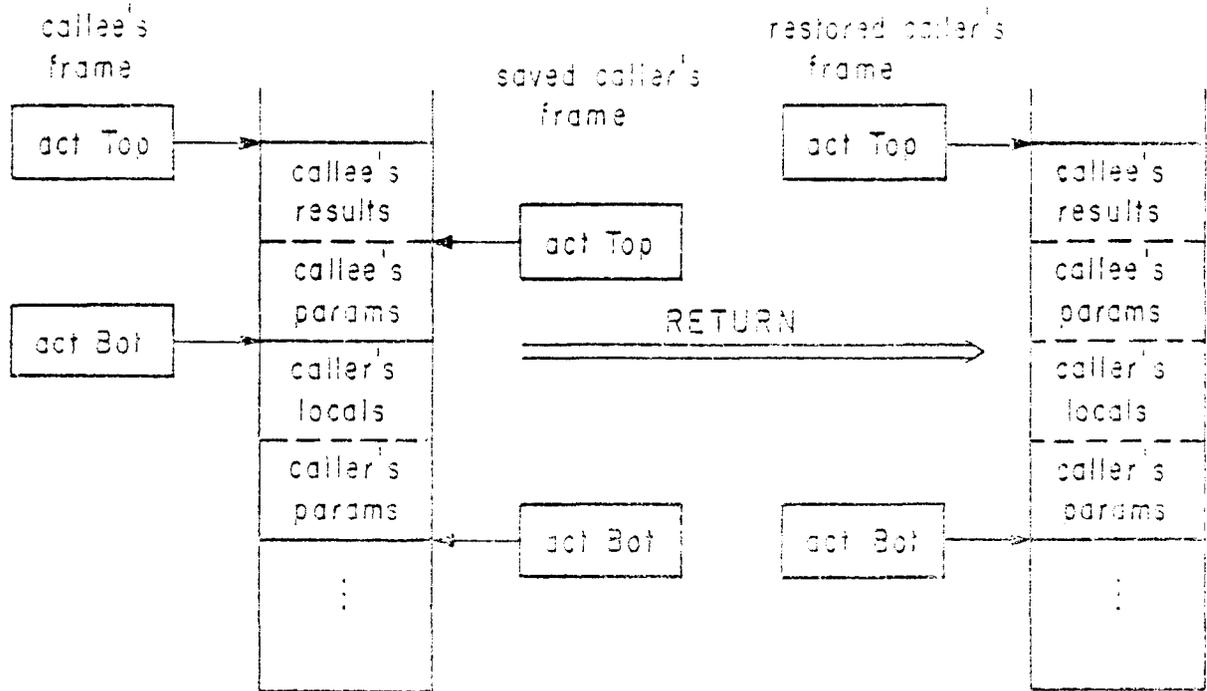
Figure 3-7: Subsystem Return -- Result Passing
