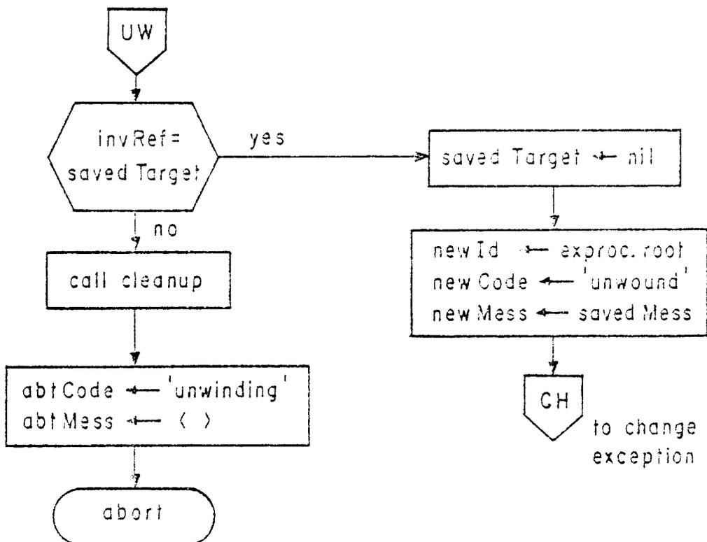
Figure 4-20: Unwind Propagation
