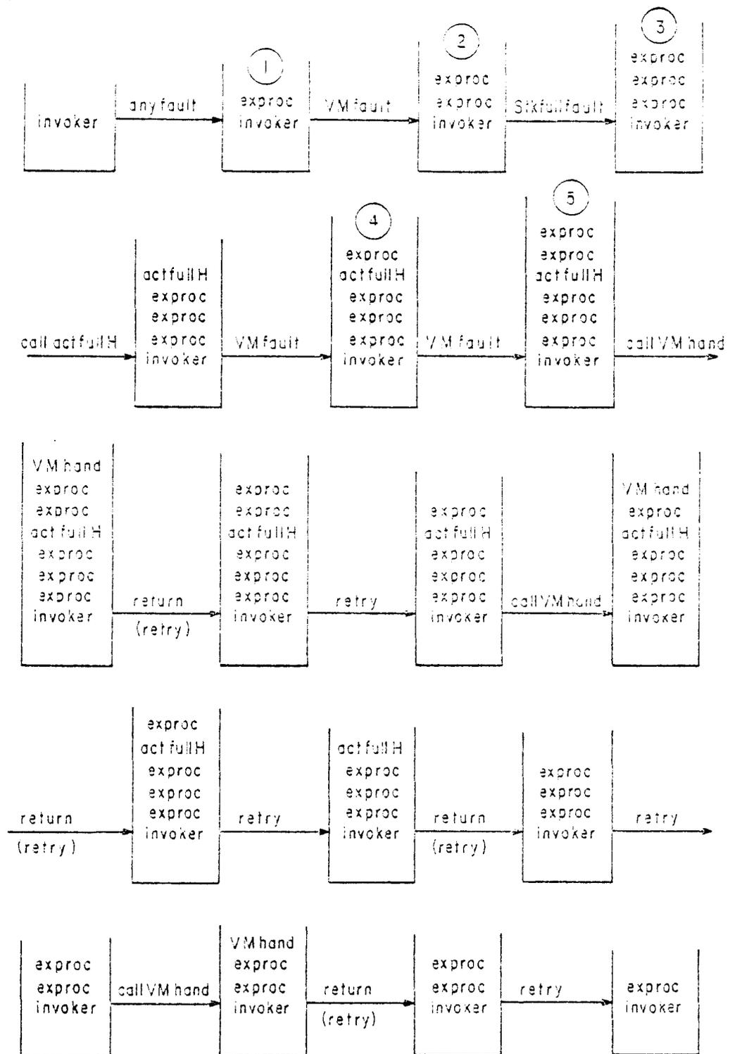
Figure 4-5: Fault Entry -- Worst Case Fault Sequence
